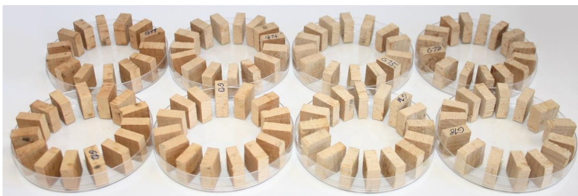
Figure 3. Samples of the hygroscopic measurements
