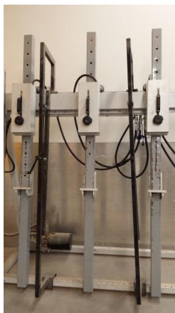
Figure 5. The Stromab STH press
