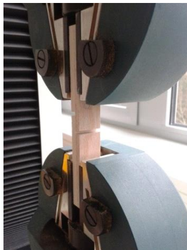
Figure 7. TiniusOlsen H10K instrument with a sample
