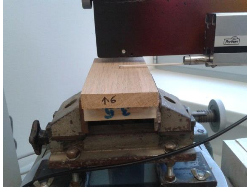
Figure 1. The S3P Perthometer with the stylus tip
