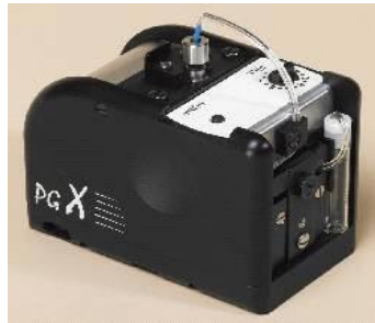
Figure 4. A PGX goniometer for surface tension measurement
