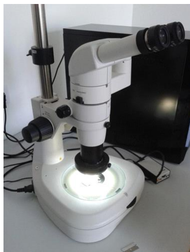
Figure 8. Nikon SMZ800 microscope
