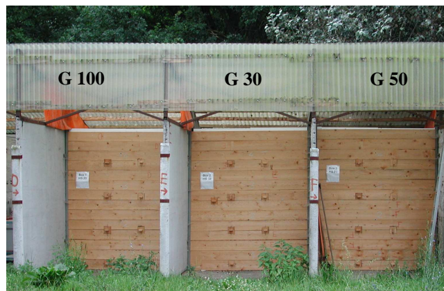
Figure 1. Storage boxes for poplar chips and chunks of different length (G 100, G 30 and G 50)
