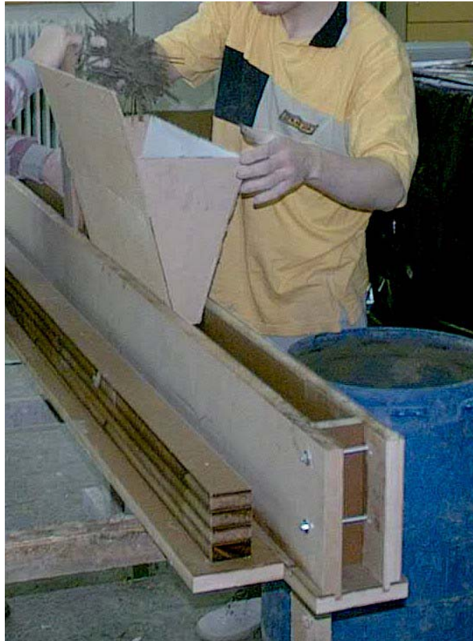
Figure 4. Aligning the strands in LSL type composites
