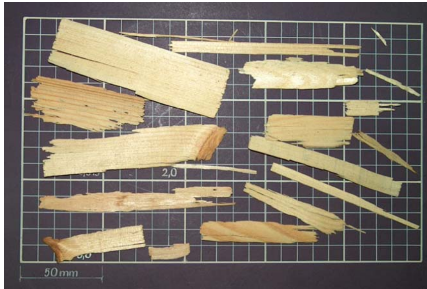
Figure 2. OSB strands used for the LSL type beams
