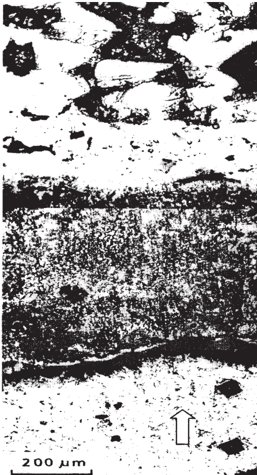
Fig. 2. Microstructure of cross-section of steel microsection after combined strengthening of LSH and SHS. A light arrow shows the direction along which the wells from the meter of the microhardness are located. The etching was carried out by nital
