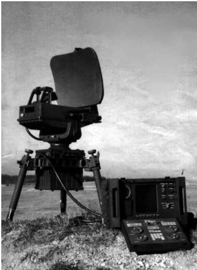
Picture 2. The RATAС reconnaissance radar station, used for the detection and display of enemy tanks and armoured combat vehicles. [5: 75]
