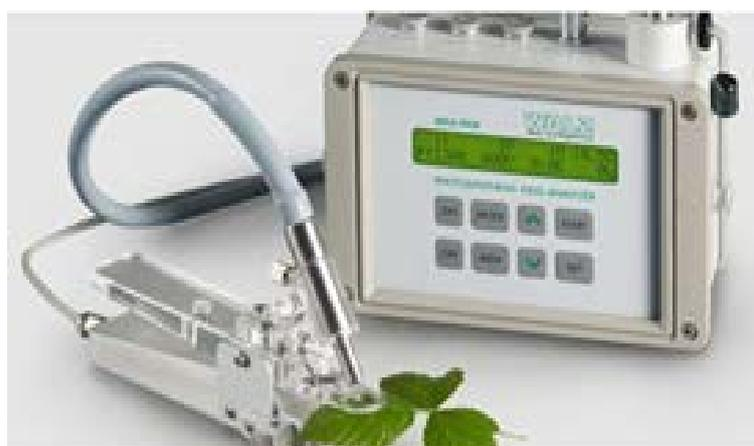
**Figure 2. MINI-PAM fluorometer**
