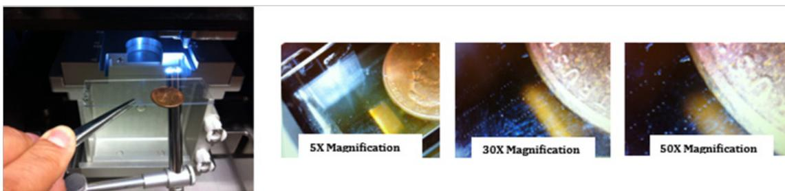
**Figure 4** Direct verification of successful drop deposition by inverted microscope with high-resolution optical lens: Andonstar Digital Microscope Video. Magnification: +100X, DSP: High Power Digital Image Monarch Processor; Sensor: high-quality CMOS sensor, 2M pixel; Resolution: 640x480, 1600x1200; Frame rate: 640x480 resolution=30 frames/sec, 1600x1200=5frames/sec; Focal distance: 5mm–30mm.
