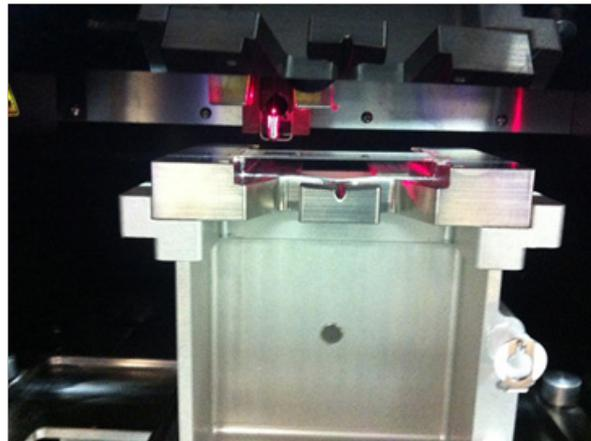
**Figure 3** Increase accuracy of single cells deposition on slide by avoiding air currents in the flow chamber, creating a vertical trajectory, re-positioning the waste stream catcher off center, and positioning the slide closer to the sorter nozzle.
