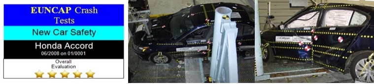
Figure 12 Honda accord 2008 EUNCAP side pole crash test [12]
