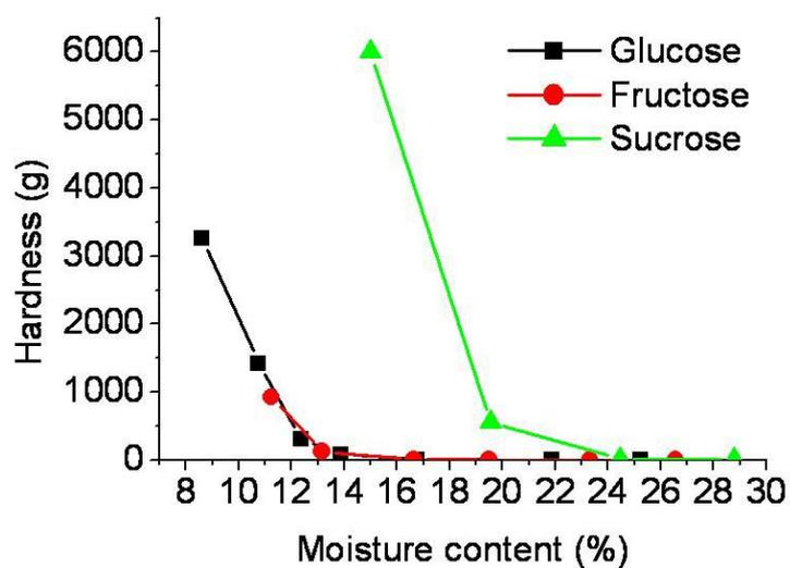
Figure 3. The dependence of hardness on the water content of glucose, fructose and sucrose solutions
