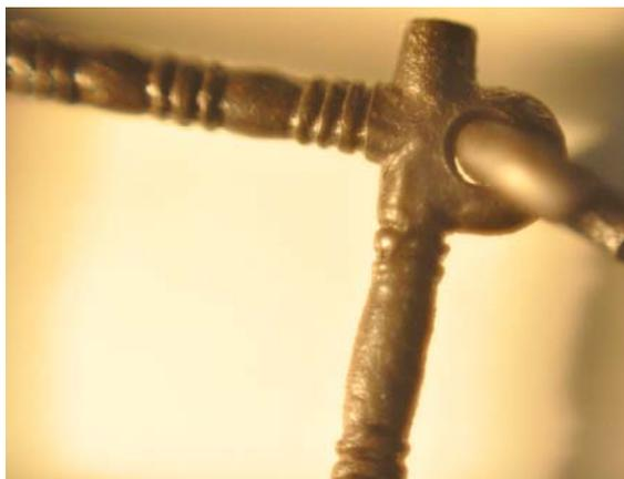
**Fig. 4.:** Magnified photograph taken from a chain fragment. The photograph reveals some details of the processing technique and shows the ornamentation of the chain.
