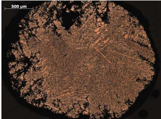
**Fig. 9.:** The microstructure of a chain fragment. Dendrites with fine secondary arms can be seen on the micrographs. Zeiss Axio Scope.A1. Magnification.: 50x. Etching: FeCl<sub>3</sub>, Bright Field
