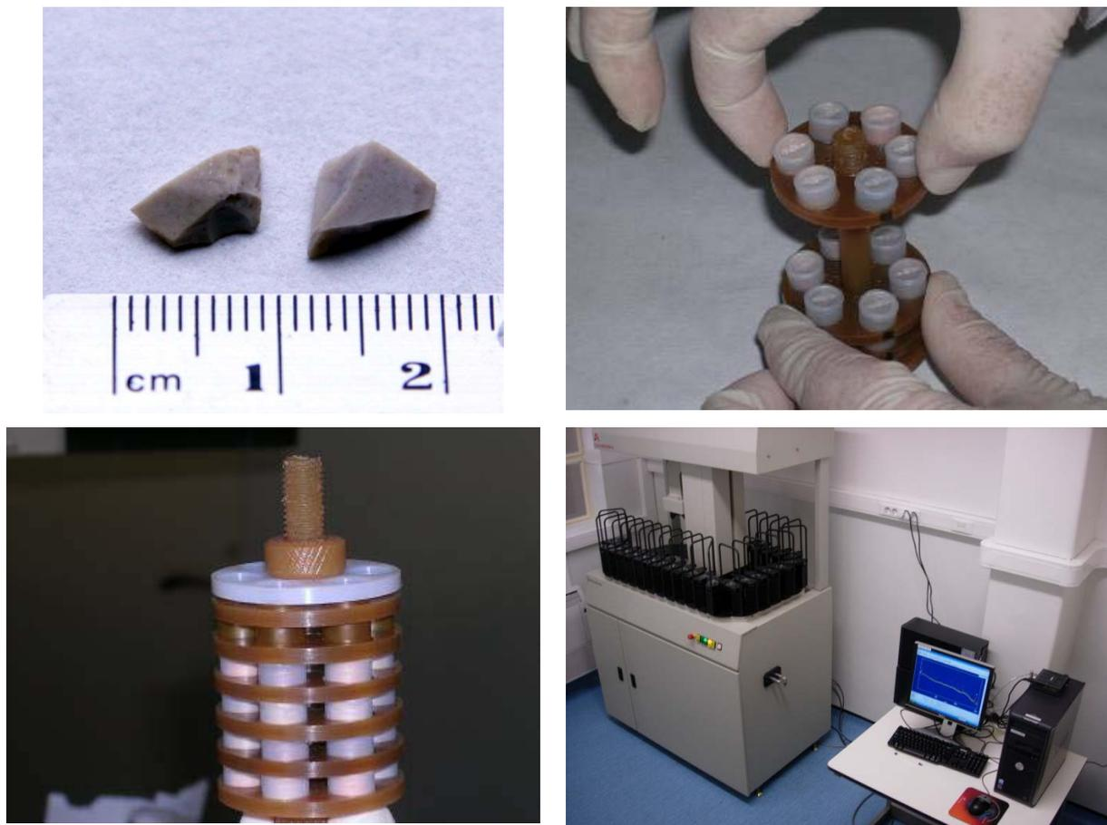
**Fig. 1.:** Photographs of: flakes of the core of a chert fragment; polyethylene vials with samples and reference samples powders; container ready to be used for long irradiations in the Portuguese Research Reactor (CTN, IST); counting room of the INAA laboratory of CTN.
