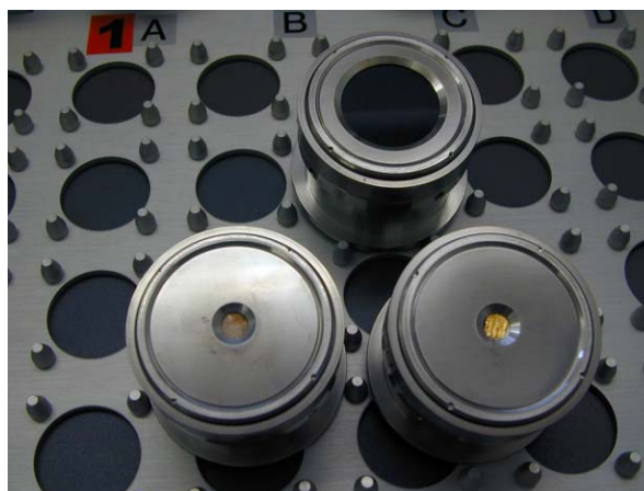
Fig. 5: Three XRF sample holders (closed, upside down), one with a conventional 34 mm window, the other two with 8 mm window, containing a rock-specimen (left) and a gold-foil (right) inside.
