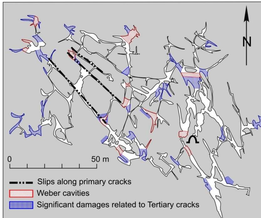
Fig. 12. Occurrences of different types of damage in western part of the Ferenc-hegy cave
