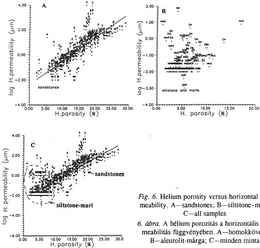
Fig. 6. Helium porosity versus horizontal permeability. A—sandstones; B—siltstone—marl; C—all samples
