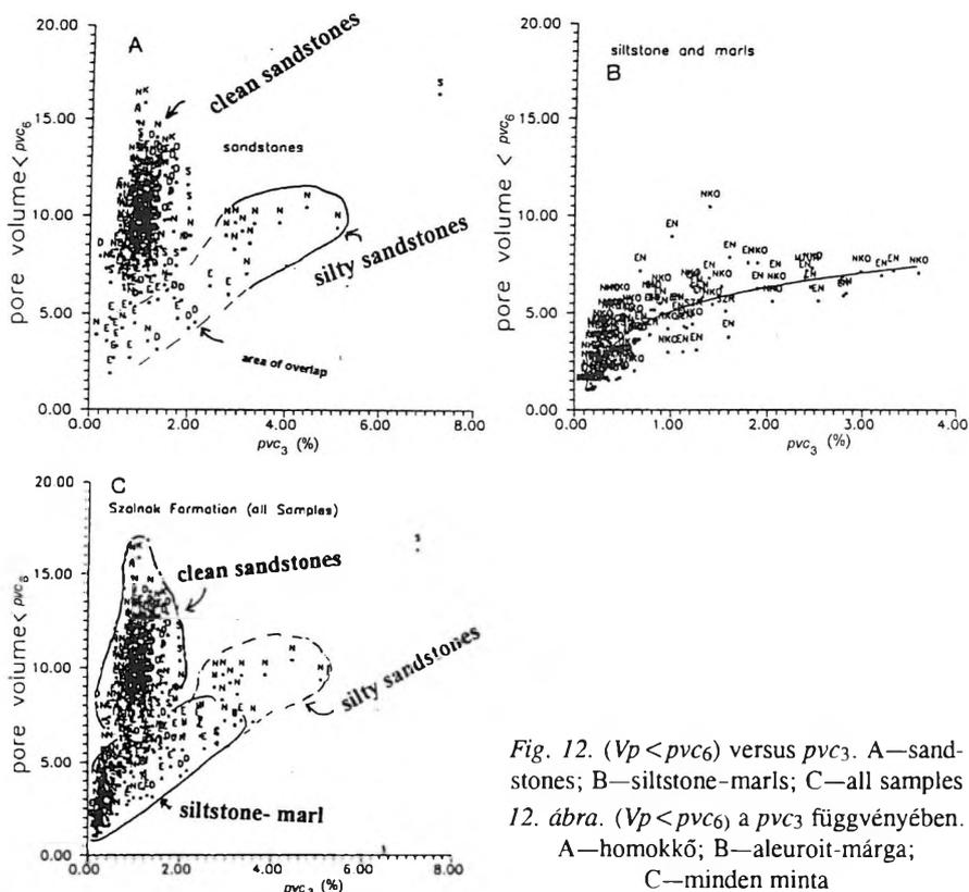
Fig. 12. ( $V_p < pvc_6$ ) versus  $pvc_3$ . A—sandstones; B—siltstone-marls; C—all samples
