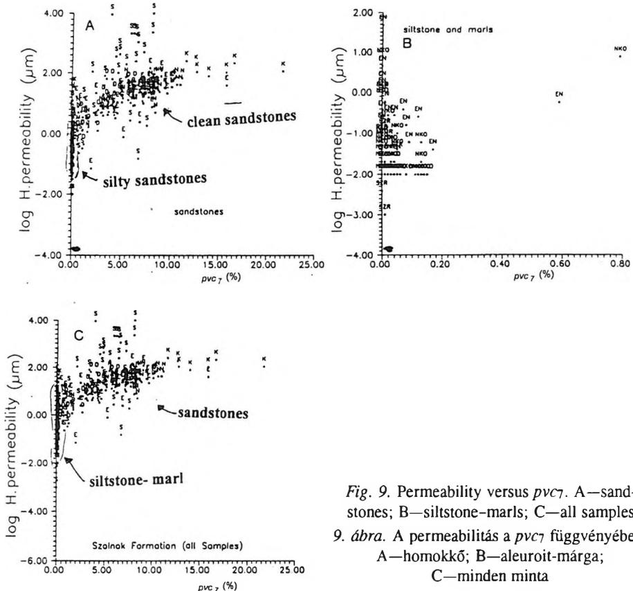
Fig. 9. Permeability versus  $pvc_7$ . A—sandstones; B—siltstone-marls; C—all samples
