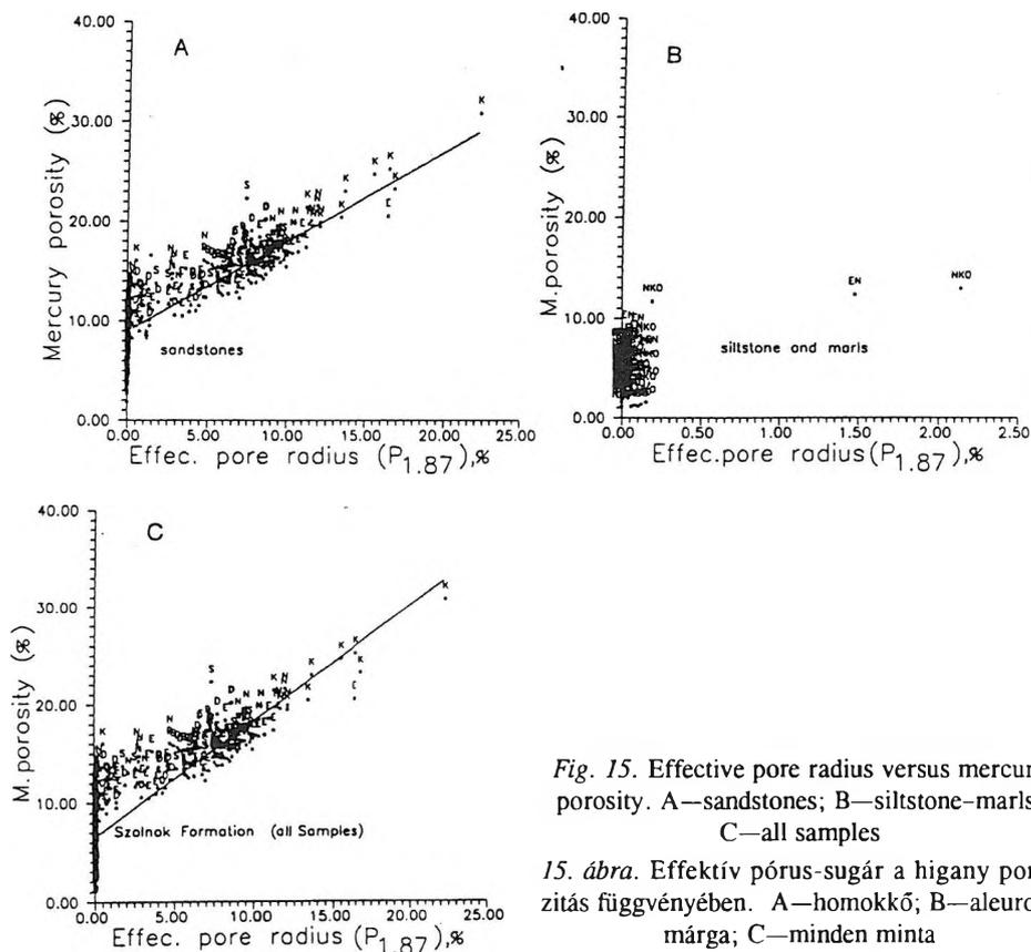
Fig. 15. Effective pore radius versus mercury porosity. A—sandstones; B—siltstone-marls; C—all samples
