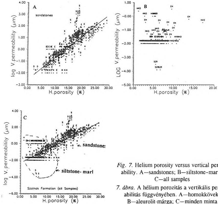
Fig. 7. Helium porosity versus vertical permeability. A—sandstones; B—siltstone-marls; C—all samples
