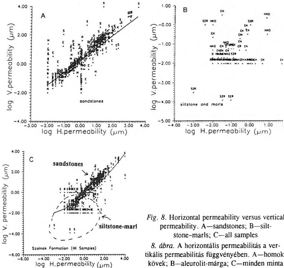
Fig. 8. Horizontal permeability versus vertical permeability. A—sandstones; B—siltstone-marls; C—all samples
