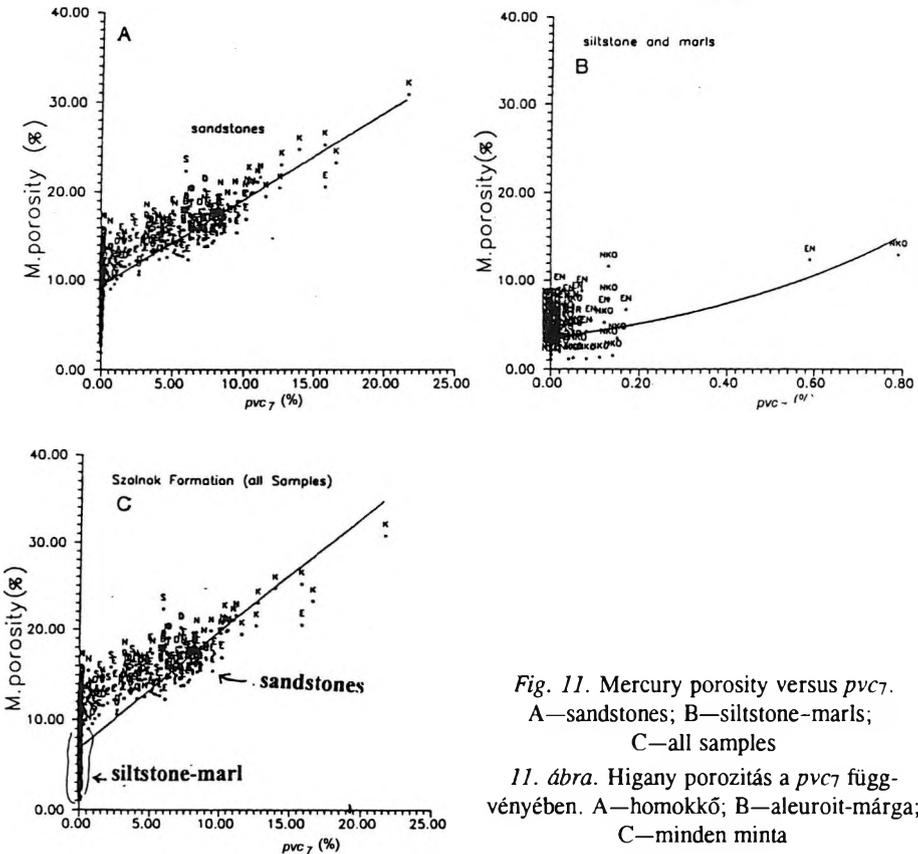
Fig. 11. Mercury porosity versus  $pvc_7$ .
