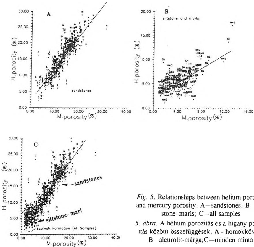
Fig. 5. Relationships between helium porosity and mercury porosity. A—sandstones; B—siltstone-marls; C—all samples
