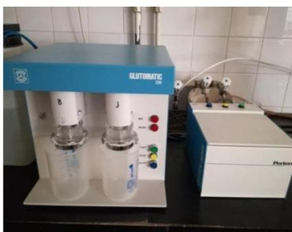
*Figure 1. Glutomatic-Gluten Index System*
